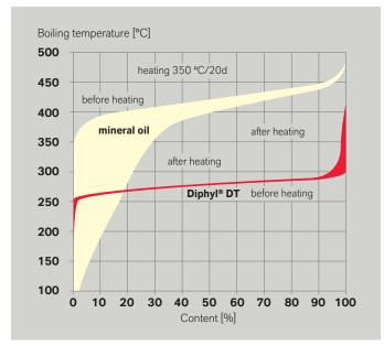
Thermal stability acc. to DIN 51528, simulated distillation GC with Diphyl® DT and mineral oil
