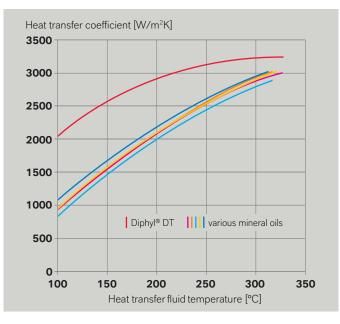
Heat transfer coefficient of Diphyl® DT compared with various mineral oils
