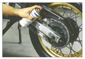
WEICON Chain and Rope Lube Spray is temperatureresistant from -40°C (-40°F) to +200°C (+392°F), strongly adherent and pressure-resistant, sound absorbent, water-resistant and has excellent creep properties. Prevents elongation, friction, and wear.
