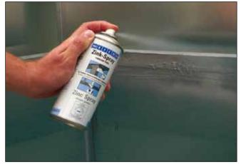
WEICON Zinc Sprays are dust-dry after about 15 minutes and can be spackled and painted over after about 12 hours without pretreatment. The temperature resistance amounts to up to  $+500^{\circ}C$  ( $+932^{\circ}F$ ) (in the case of "bright grade", up to  $+300^{\circ}C$  /  $+572^{\circ}F$ ).
